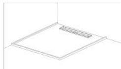
5. Fill and keep the ground to tilt 1-2°
