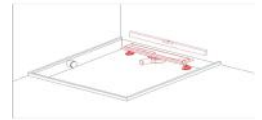
3. Put the shower drain in place and use spirit-level to ensure the horizontal surface around it.
