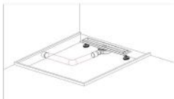
4. Install the water pipes
