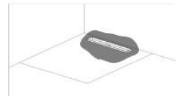
6. Brush the first waterproof coating
